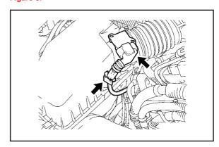
D. Loosen the hose clamp and air cleaner cap with air cleaner hose.
