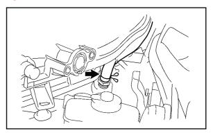
E. Remove the bolt and water hose joint from the intake air surge tank.
