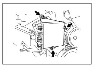
26. Remove the timing chain cover plate by removing the 4 bolts, timing chain cover plate, and timing chain cover plate gasket.
