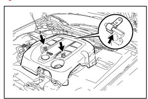
B. Raise the cover again to remove the 2 nuts on the front of the cover and remove the cover.
