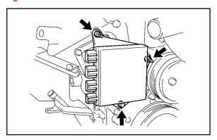
10. Install the No. 1 engine cover with the 3 clips.
