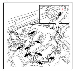
C. Install the bolt and 2 nuts to the intake air surge tank.
