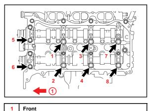
(6) Tighten the 8 M6 bolts to their final torque value in the sequence shown in Figure 50. Torque: 16 N\*m (163 kgf\*cm, 12 ft\*lbf)
