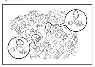
(2) Uniformly loosen and remove the 9 camshaft bearing cap M6 bolts in the sequence shown in the illustration.
