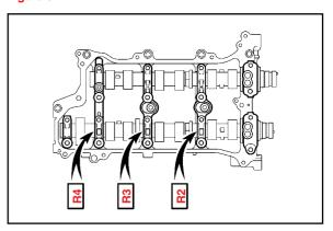
(4) Tighten the 9 M6 bolts in the sequence shown in the illustration.
