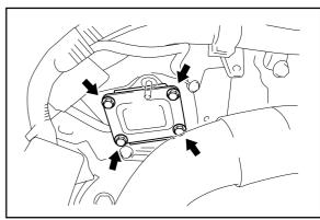
9. Install the injector driver with the bolt and 2 nuts. Torque: 10 N\*m (102 kgf\*cm, 7 ft\*lbf)
