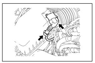
26. Connect the ventilation hose from the cylinder head.
