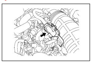
C. Connect the MAF meter connector and clamp to the air cleaner.
