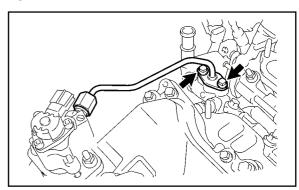
B. Using a 19-mm union nut wrench, connect the fuel pipe.
