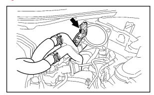
F. Connect the ventilation hose to the intake air surge tank.
