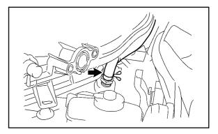
G. Connect the wire harness and hose to the intake air surge tank.
