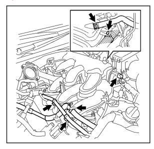
D. Disconnect the ventilation hose from the intake Figure 16. air surge tank.
