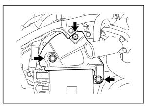
25. Remove the injector driver by removing the bolt and 2 nuts.
