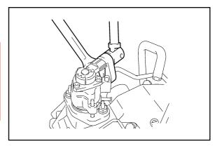
C. Remove the 2 bolts on the delivery pipe side.
